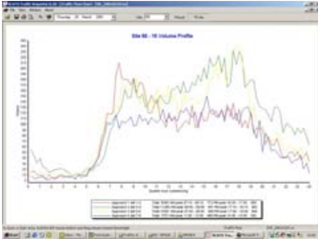
Volumes data is collected from all lanes at all junctions 24 hours a day.
