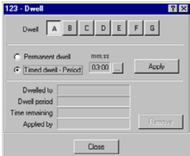
A dwell manually forces the controller to the nominated stage via the shortest possible path, subject to all safety constraints being met and to remain there for a fixed period.
