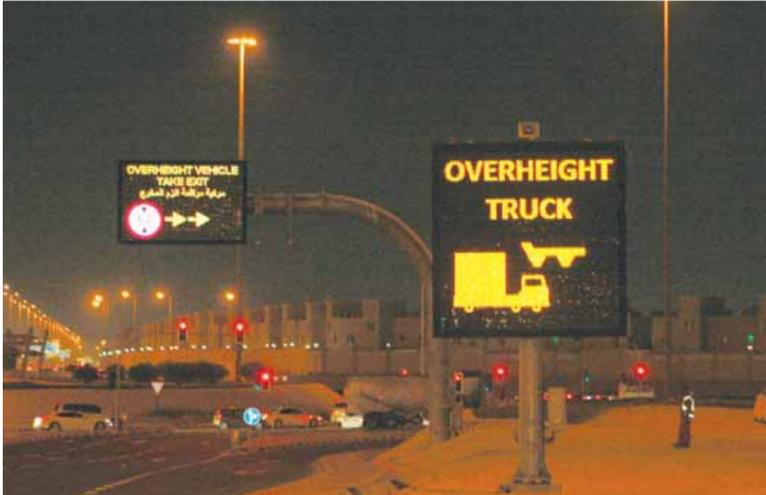
The OVDWS sensors and the display boards installed in Gharaffa on the Shamal-Doha Expressway's entry point towards Duhail interchange. PICTURE: Shaji Kayamkulam
